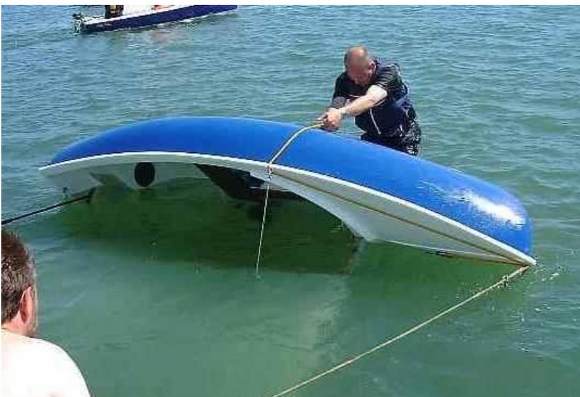
Here the painter can be seen led inside a shroud. As the rig emerges from the water the scow should right rather quickly. The crew should then climb aboard from his/her position at lowest part of the side.
