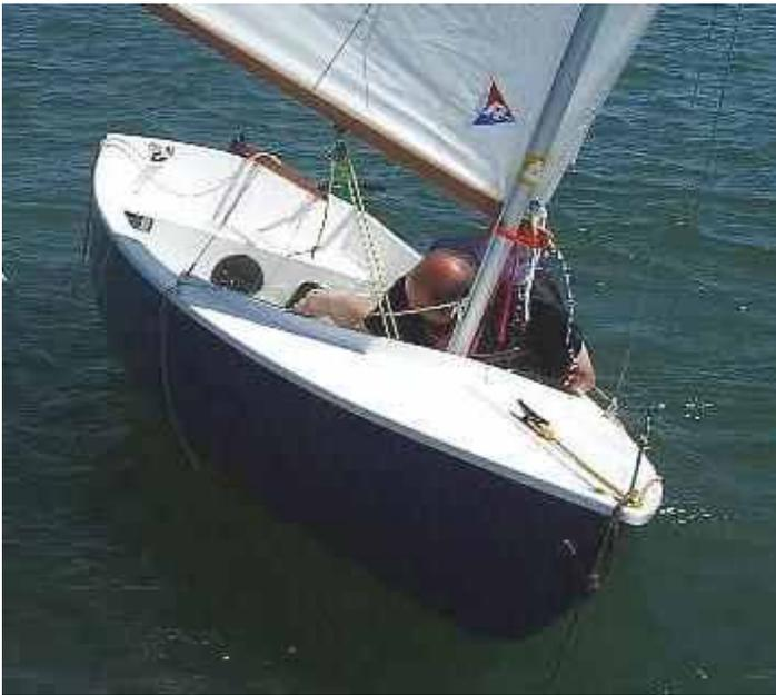
The scow will right with a good bathfull of water in the cockpit. This can be bailed out in 2-3 minutes with a normal dinghy bailer. Even with this water aboard the scow remains remarkably stable. The following picture shows that even when an 80kg crew sits at one side there is still around 10cm freeboard on the low side.
