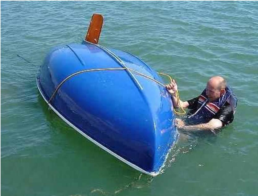
This starts the righting process. The gunwhale on the crew's side can be immersed further if the crew puts his/her feet on the underside of the gunwhale whilst maintaining tension on the painter.
